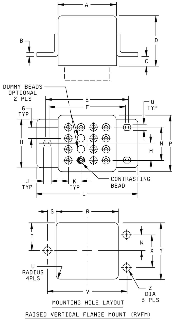
FIGURE 1. Dimensions and configurations - Continued.
